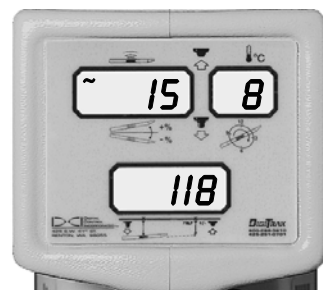
Tracking Mode Showing Pitch, Roll, Depth/Distance, and Update Symbol
